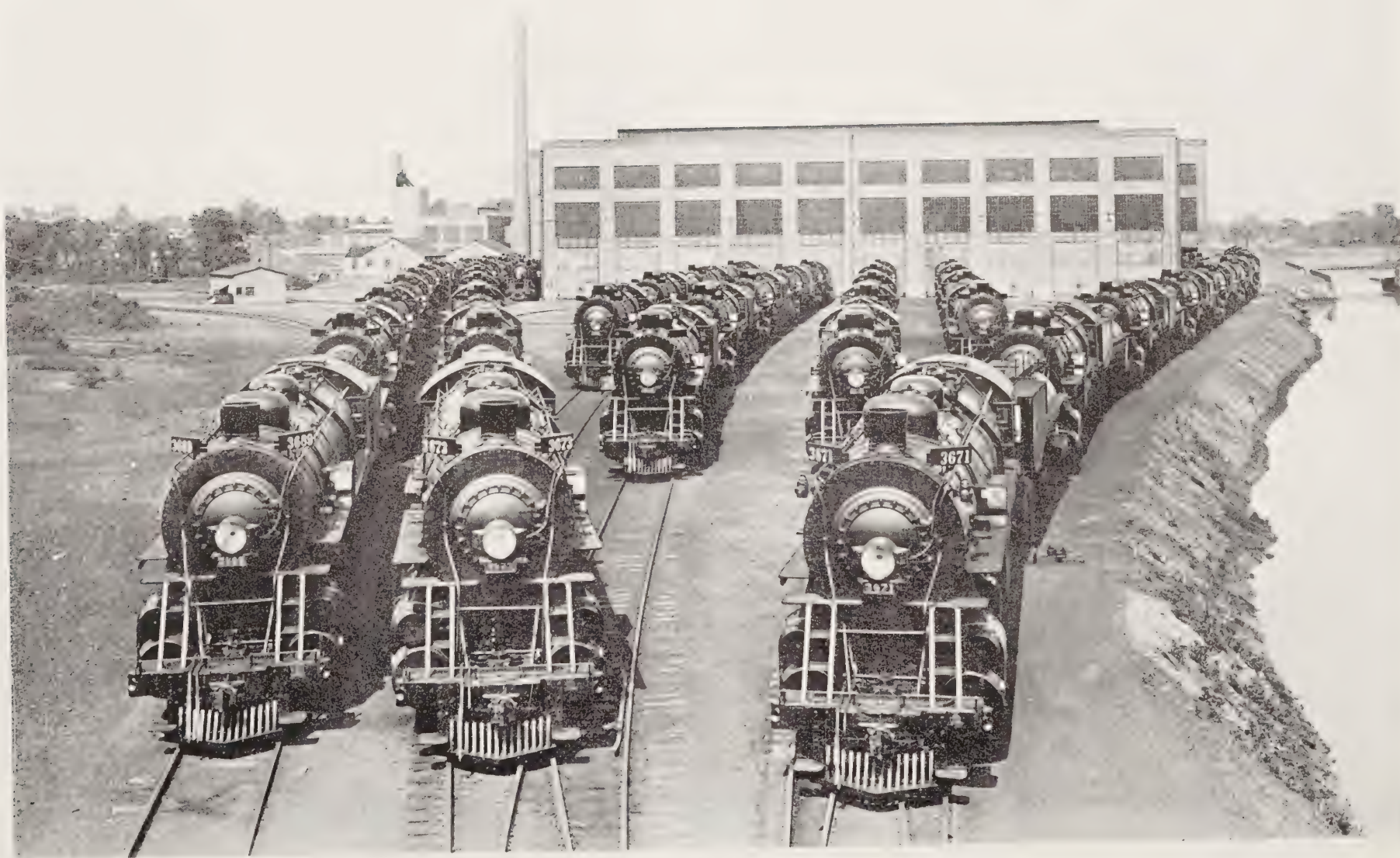
Fifty 2-10-2 Type Locomotives for the Southern Pacific Lines Ready for Shipment from the Eddystone Plant of The Baldwin Locomotive Works.
